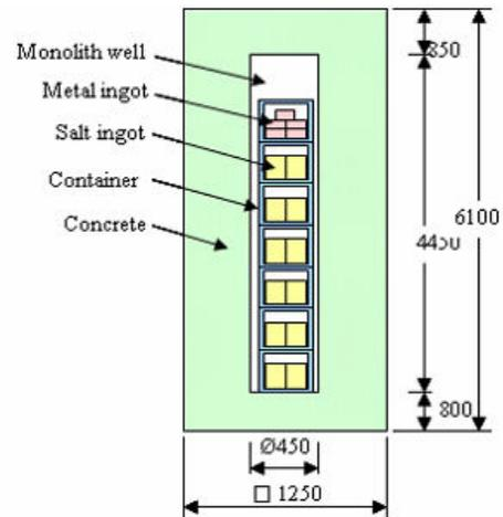
Fig. 4. Monolith Storage Model.
