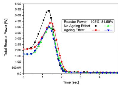
Figure 1. Total reactor power at 81.59 & 103% FP
