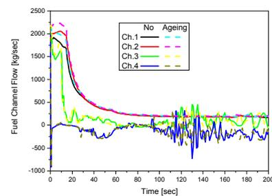
Figure 2. Fuel channel flow at 81.59% FP
