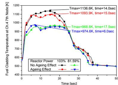
Figure 3. Fuel cladding temperature at 81.59 & 103% FP
