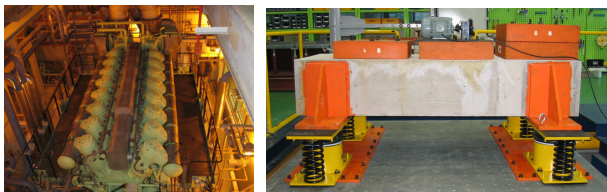
(a) Target EDG System (b) Scaled Test Model Fig. 1 Emergency Diesel Generator
