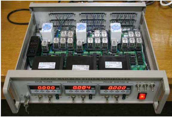
Figure 3. Upgraded control circuit of the DLSTS.
