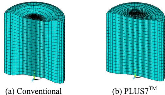
Figure 2. Finite Element Models for Stress Analysis
