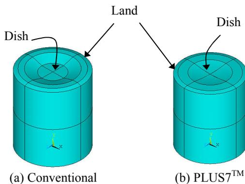
Figure 1. Morphology of conventional and PLUS7  $UO_2$  pellets
