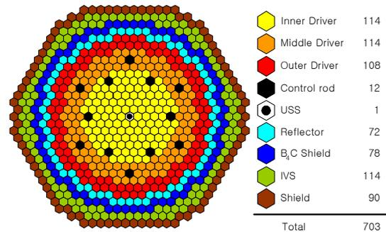
Figure 1 Core configuration
