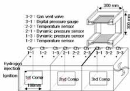
Fig. 1 Combustion Chamber
