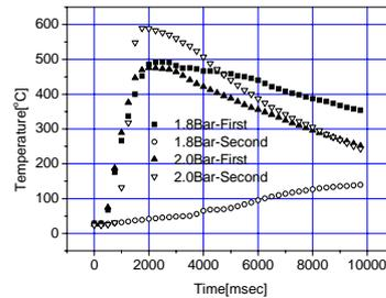
Fig. 3 Compartment gas temperature during burn
