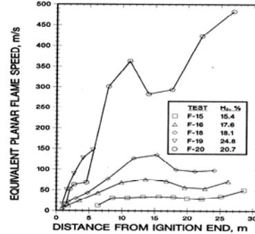
Fig. 7 Comparison of flame speeds for tests with 13% top venting and no obstacles[9]
