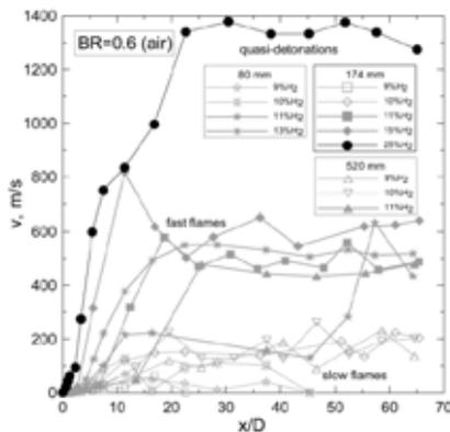
Fig. 6 Propagation speed of flames and detonation along the tube vs ratio of distance,  $x$ , tube diameter,  $D$ [8]
