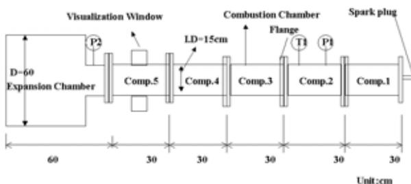
Fig. 2 Combustion chamber for a high flame speed
