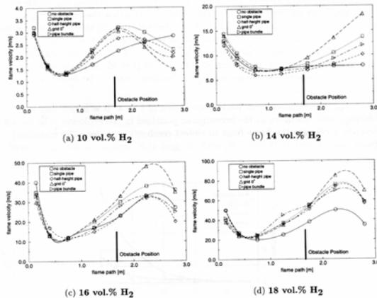
Fig. 5 Flame speed vs. flame path for obstacles[7]
