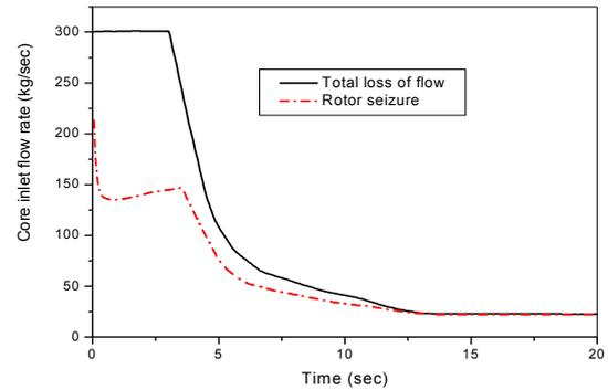
Figure 1. Core inlet flow rate of loss of coolant flow accidents.
