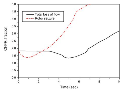
Figure 2. CHF behavior of loss of coolant flow accidents.
