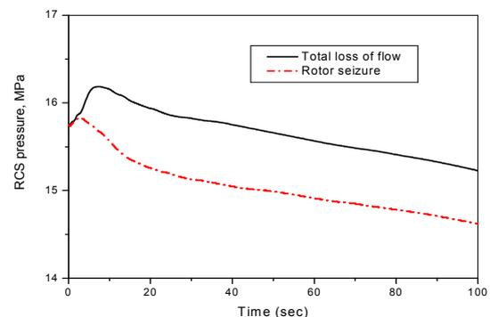
Figure 3. RCS pressure of loss of coolant flow accidents.
