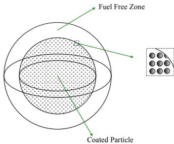
Figure 2. A model for doubly heterogeneous pebbles
