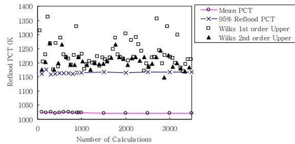
Figure 1. Comparisons of 95% upper reflood PCTs with limit value of Wilks' formula
