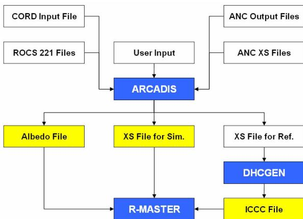
Figure 1. The procedure to generate the simulator core model
