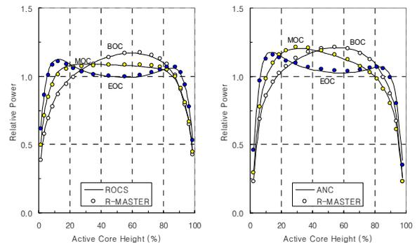
Figure 2. Comparison of axial power distribution of Ulchin unit 3 cycle 7 and Younggwang unit 1 cycle 16 (HFP, ARO)
