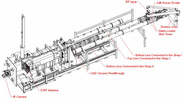
Figure 2. 3-D drawing of the test stand for RF test campaign-9
