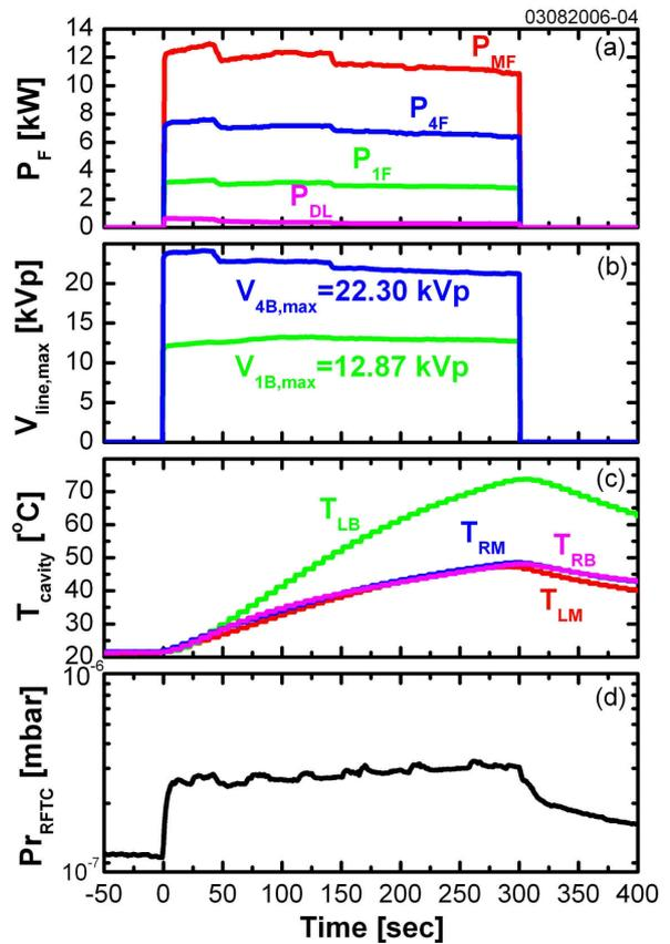
Figure 4. Time evolutions of the RF powers (a), line voltages (b), temperatures of the antenna cavity (c), and vacuum pressure of the RFTC (d) measured during 300-s long-pulse duration.
