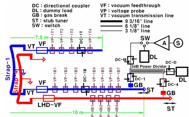
Figure 1. Schematic diagram of the two-strap feeding test circuit for the RF test campaign-9.
