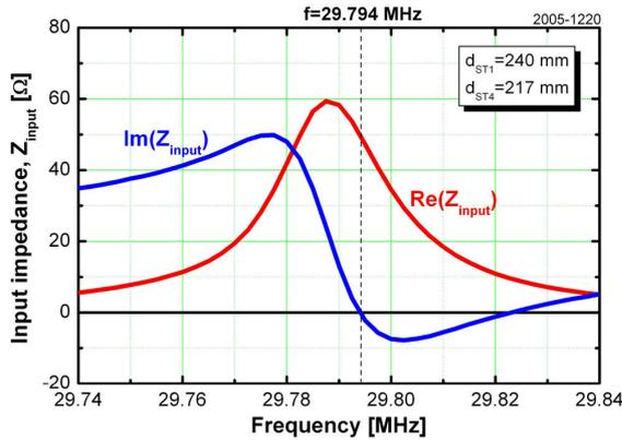
Figure 3. Measured input impedance of the test circuit.
