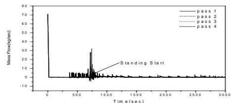
Fig.2 Coolant flow rate after the failure of SDCS pumps
