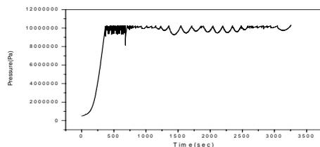
Fig.3 Pressure of the coolant in the ROH
