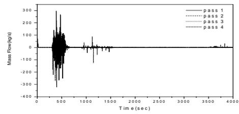
Fig.8 Coolant flow rate after SG manway open
