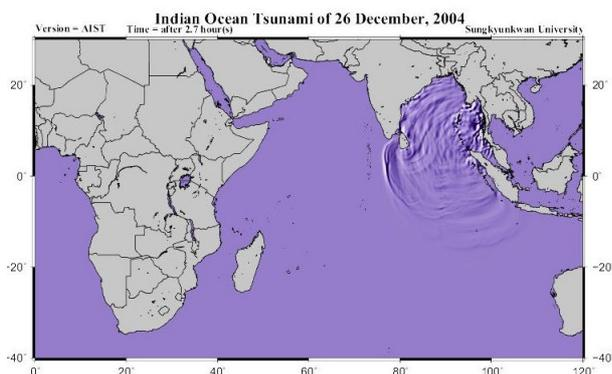
Figure 1. Snapshot of modeled tsunami propagation 2.7 hours after the earthquake
