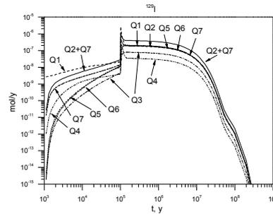
Fig. 5. Release of  $^{129}\text{I}$  from seven exit points to the single fractures or fracture zones in the near-field of the repository.
