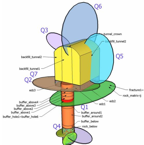
Fig. 1. Near-field of the repository embedded by fractures.
