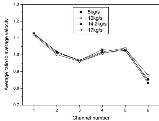
Figure 3. Averaged velocity distribution in each channel of tubular fuel
