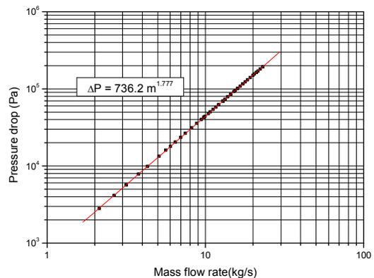
Figure 4. Pressure drop with changing of mass flow rate
