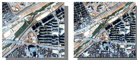
4m × 4m resolution 16m × 16m resolution Fig. 1. Images Comparison (Spatial Resolution)
