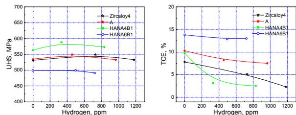
Fig. 1. Burst properties of cladding tube specimens with the change of hydrogen content at 350 °C
