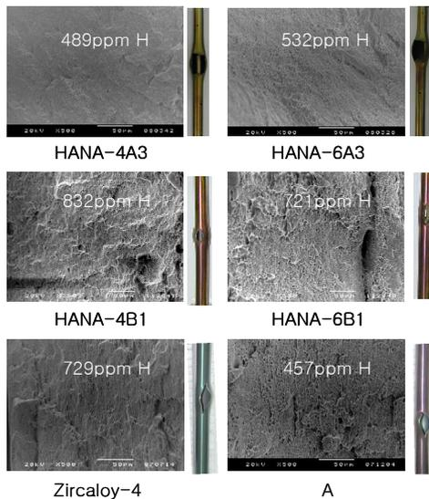
Fig. 3. Fractographs of the hydrided specimens (x500)
