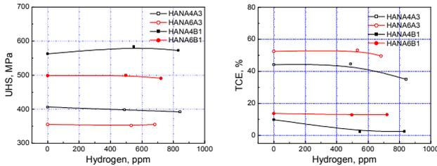
Fig.2. The effect of hydrogen and final heat treatment on the burst properties of HANA cladding tube specimens at 350°C
