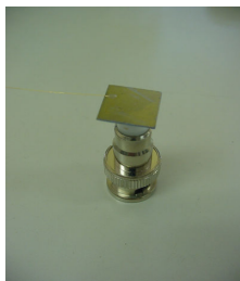
Figure1. Photos of the fabricated SI-GaAs bulk diode structure detector.
