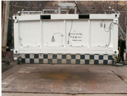
Figure 1. The top-vertical drop test of the IP-2-a transport package.
