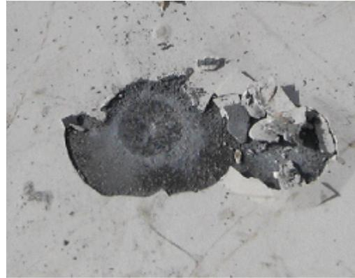
Figure 3. Deformation at the impact area for a penetration test of the type A transport package.
