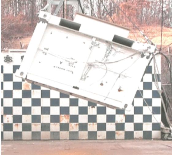
Figure 2. The top-oblique drop test of the type A transport package.
