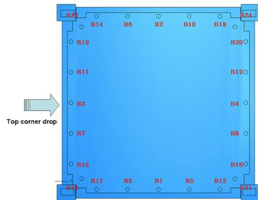
Figure 1. The order of the fastening bolts for top-oblique drop of the type A transport package.
