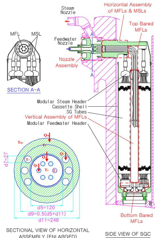
Fig. 1. The SGC with a Sectional View of the Horizontal Assembly of the MFLs and MSLs
