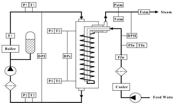
Fig. 2. Schematic Diagram of SG Test Facility
