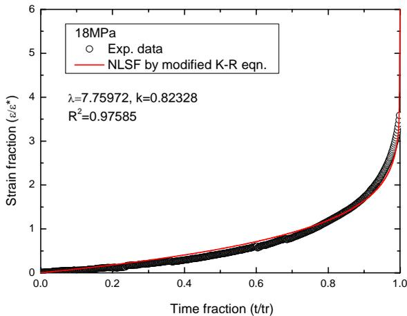
Figure 4. Comparison between the experimental data and NLSF of the modified equation at 18MPa.
