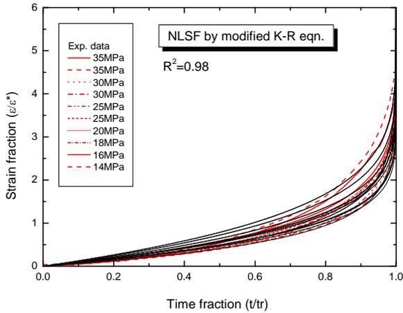
Figure 3. Strain fraction vs. time fraction by NLSF of the modified equation.
