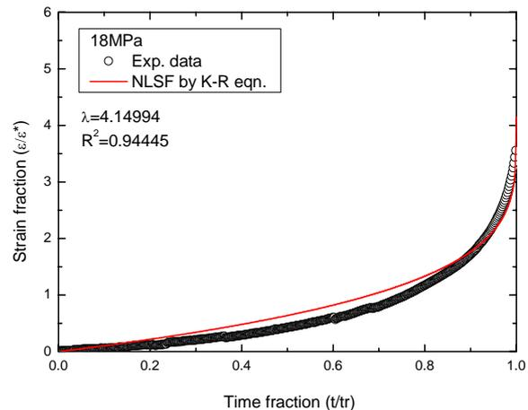
Figure 2. Comparison between experimental data and NLSF of K-R equation in 18MPa.
