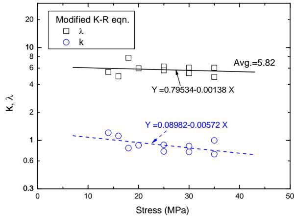
Figure 5. The  $K$  and  $\lambda$  variations as a function of the stress by the modified eqn..
