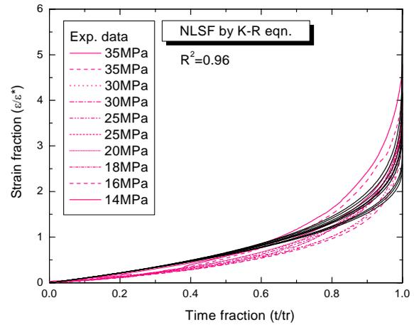
Figure 1. Strain fraction vs. time fraction by NLSF of the K-R equation.
