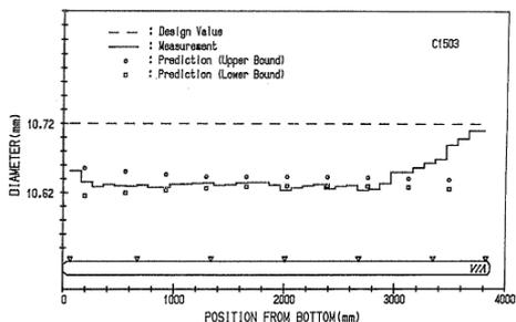
Figure 2. Diameters of nuclear fuel rod of three burnup cycles.
