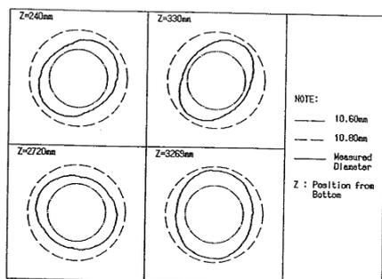
Figure 5. Ovalities on location of nuclear fuel rod of two burnup cycles.
