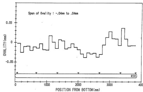
Figure 6. Ovalities of nuclear fuel rod of three burnup cycles.
