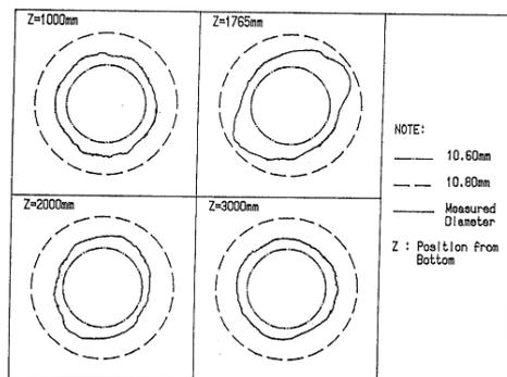
Figure 7. Ovalities on location of nuclear fuel rod of three burnup cycles.
