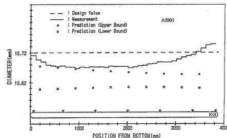
Figure 1. Diameters of nuclear fuel rod of two burnup cycles.
