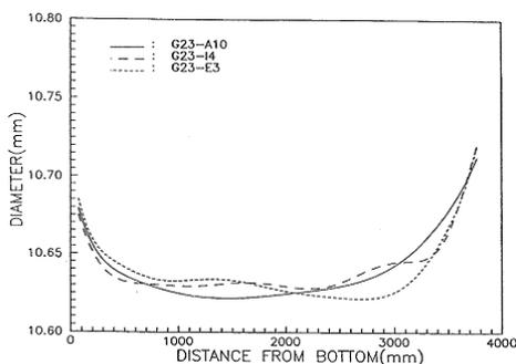
Figure 3. Diameters of nuclear fuel rod of four burnup cycles.
