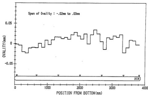
Figure 4. Ovalities of nuclear fuel rod of two burnup cycles.
