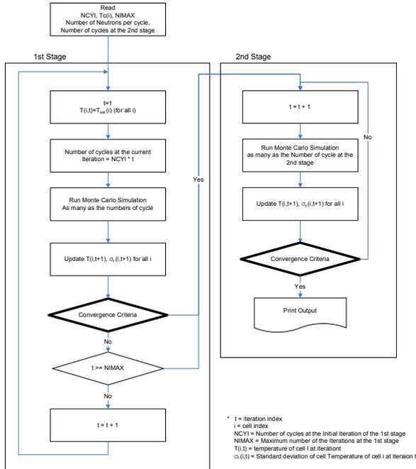
Figure 1. Flowchart of iterative MC neutronics calculation with thermal hydraulic feedback.
