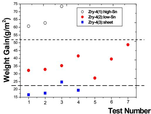
Figure 3. The weight gains at 800°C, 10MPa steam.
