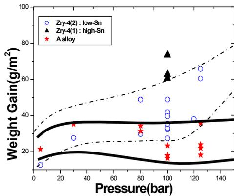
Figure 2. The weight gain versus steam pressure at 800°C.
