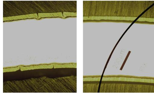
Figure 4. Cross sectional view of specimens oxidized at 800°C, 10.0MPa (Left : high-Sn Zry-4, Right : low-Sn Zry-4)
