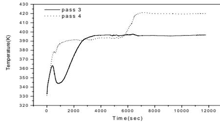
Fig.9 Fuel sheath temperature during the TS with one SG/loop fed
