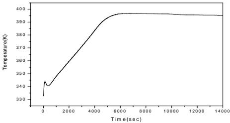
Fig.6 Fuel sheath temperature during the TS
