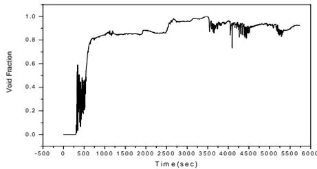
Fig.1 Coolant void fraction after the loss of SDCS
