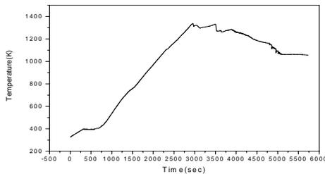
Fig.2 Fuel sheath temperature after the loss of SDCS
