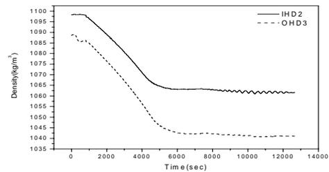
Fig.3 Coolant densities of RIH & ROH due to the TS
