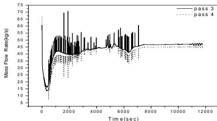
Fig.7 Coolant flow rate during the TS with one SG/loop fed
