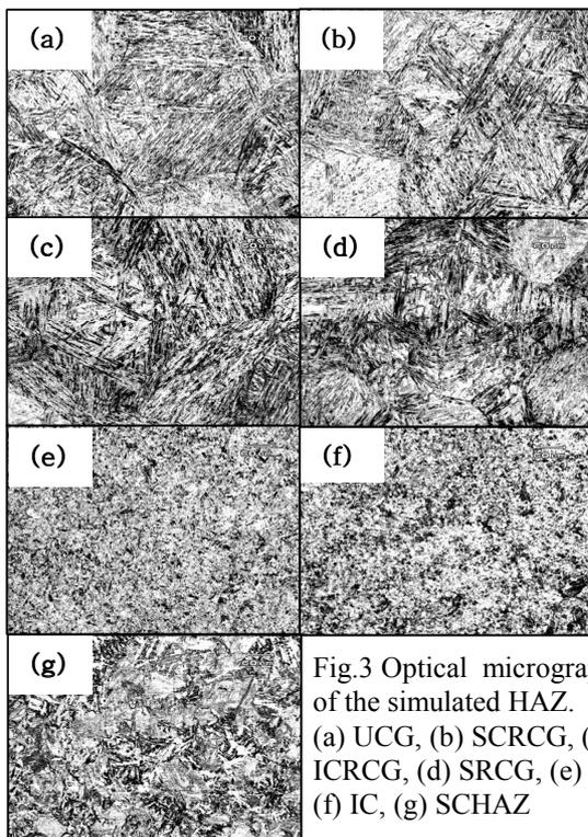
Fig.3 Optical micrographs of the simulated HAZ. (a) UCG, (b) SCRCG, (c) ICRCG, (d) SRCG, (e) FG, (f) IC, (g) SCHAZ
