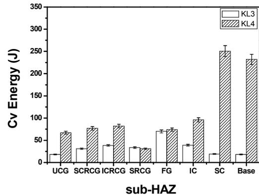
Fig.4 Charpy impact test results of various sub-HAZ at -29°C
