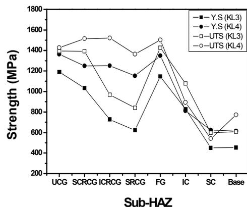
Fig.1 Yield and tensile strength of simulated HAZ (KL3, KL4)
