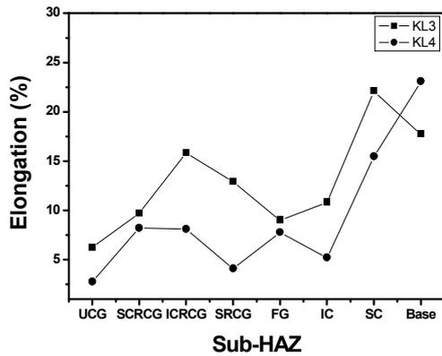
Fig.2 Elongation results of simulated HAZ.
