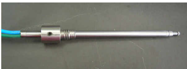
Figure. 3 Fixing Device Combined with a Sensor for Remote Precision Measurement
