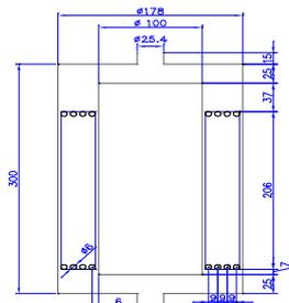
Figure 1. Test section for 2 components heat exchanger system
