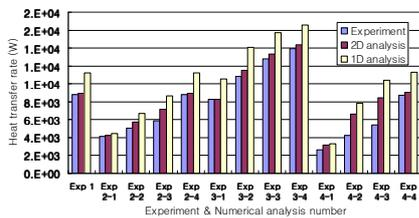
Figure 2. 2 component normal system heat transfer rate
