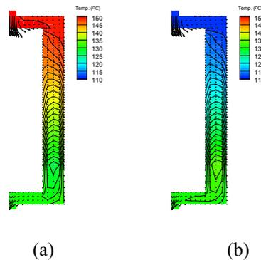
Figure 6. Shell side temperature distribution
