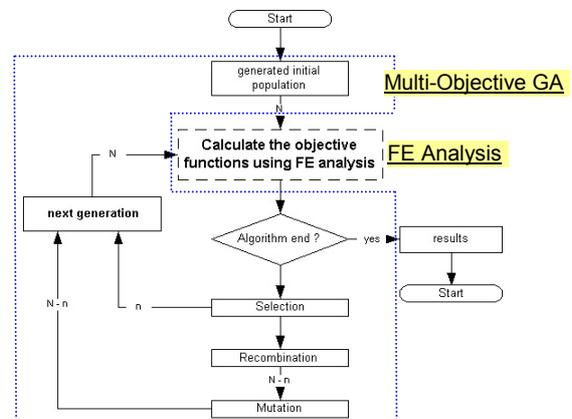
Figure 1. General scheme of the FE analysis and the multi-objective GA
