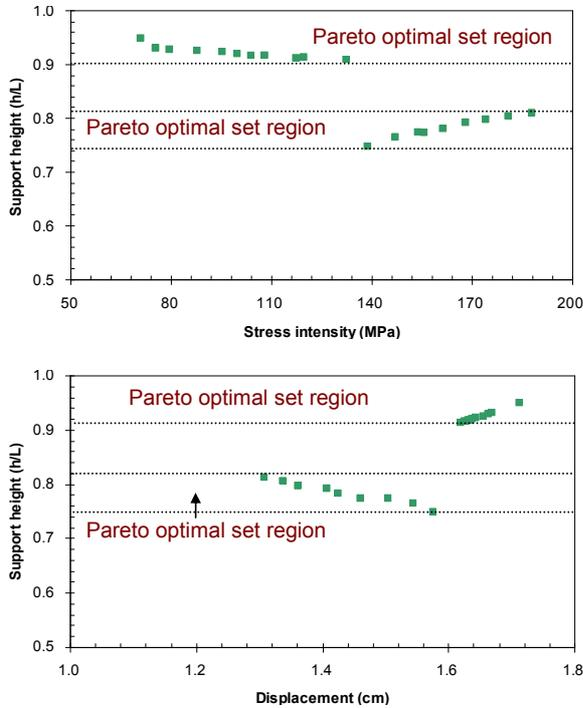
Figure 3. Stress intensities and displacements for support height variation
