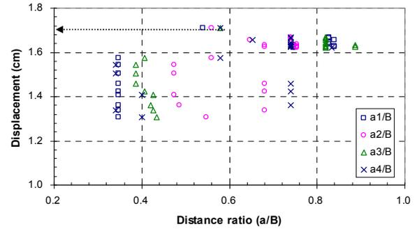
Figure 4. Stress intensities and displacements by depending on support distance ratios ( $a/B$ )
