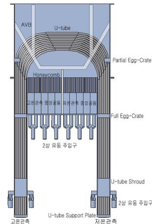
Figure 1. Schematic of test section (front view)
