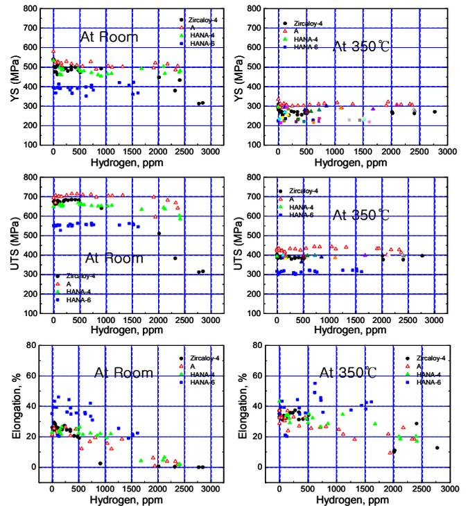
Fig.2. Circumferential mechanical properties of claddings at both room temperature and 350 °C with the change of hydrogen content
