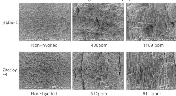
Fig.3. fracture surfaces of HANA-4 and Zircaloy-4 claddings at room temperature
