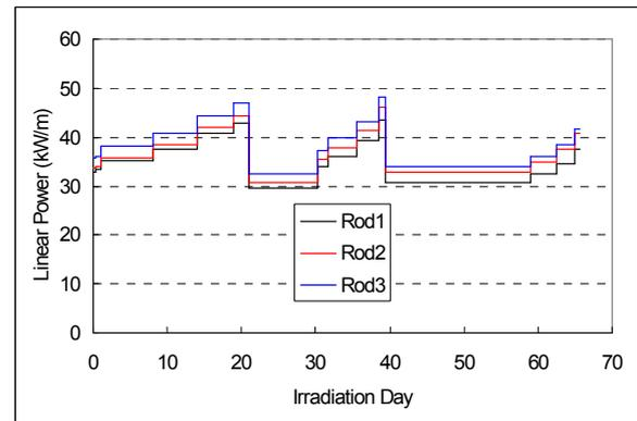
Figure 1. Linear power change during the fifth irradiation test of the dry process fuel.
