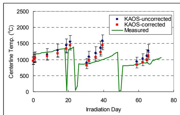
Figure 3. Centerline temperature distribution of uncorrected and corrected results for the sixth irradiation test of the DUPIC fuel.
