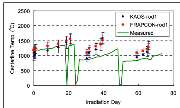
Figure 2. Centerline temperature distribution for the sixth irradiation test of the DUPIC fuel.
