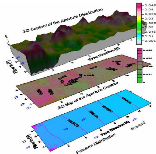
Fig.1 Aperture distribution of the granite core.
