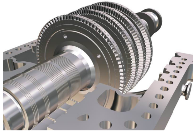
Figure 1. Rotor and blade of four stages gas turbine.
