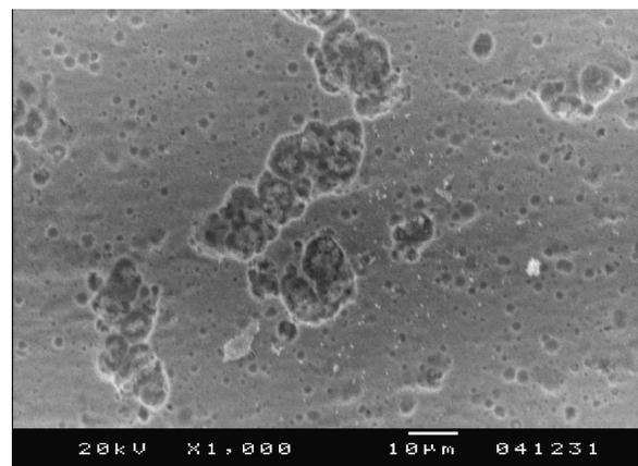
Figure 1 SEM photographs of the inner surface after test in a 350°C 280 MPa iodine environment.
