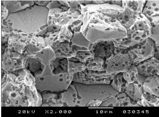
Figure 2 ISCC Fracture surface of the Zircaloy-4(RX) pressurized in an iodine environment.
