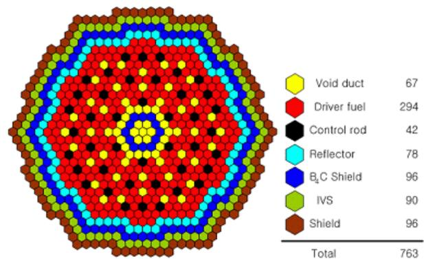
Figure 1. Transmutation core using void ducts
