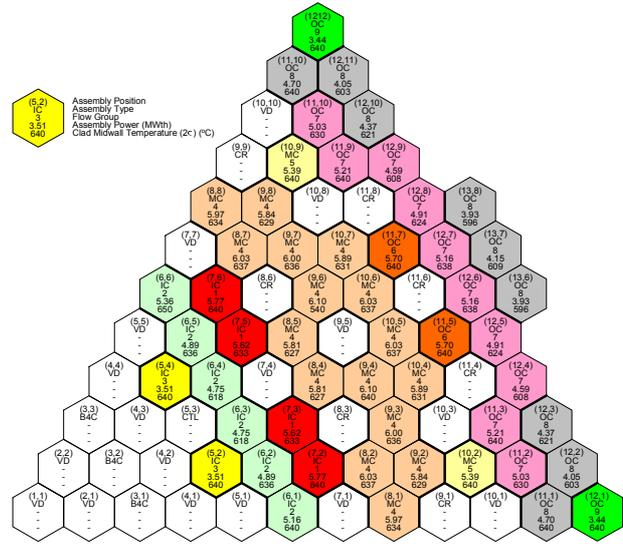
Figure 2. Flow groups and cladding midwall temperatures ( $2\sigma$ ) (1/6 Core)
