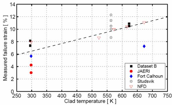
Figure 1. Clad failure strain vs. temperature for un-irradiated claddings with negligible hydrogen content, tested at low strain rate. Filled symbols: Zircaloy-4. Open symbols: Zircaloy-2.
