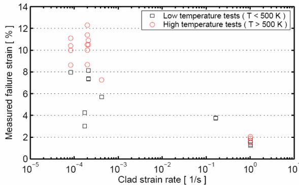
Figure 2. Clad failure strain vs. hoop strain rate for un-irradiated cladding with negligible hydrogen content (<15 ppm).
