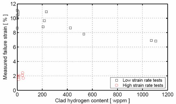
Figure 5. Clad failure strain vs. hydrogen content, determined from tests on un-irradiated cladding at temperatures between 523 and 673 K at low (<math>10^{-3} s^{-1}</math>) and high hoop strain rate (>math>10^{-1} s^{-1}</math>).
