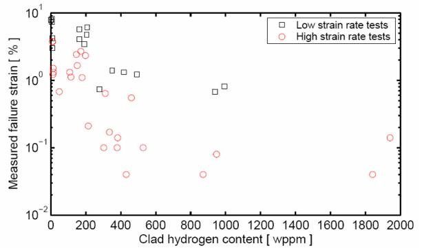
Figure 4. Clad failure strain vs. hydrogen content determined from tests on un-irradiated cladding at room temperature at low (<math>10^{-3} s^{-1}</math>) and high hoop strain rate (>math>10^{-1} s^{-1}</math>).
