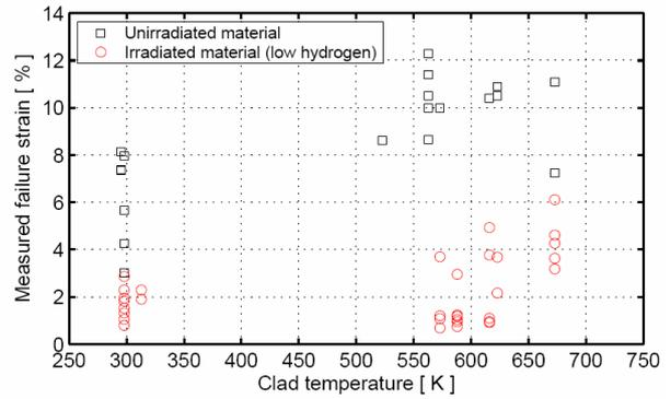
Figure 3. Clad failure strain vs. temperature for un-irradiated and irradiated claddings at low hoop strain rate (<math>10^{-3} s^{-1}</math>).
