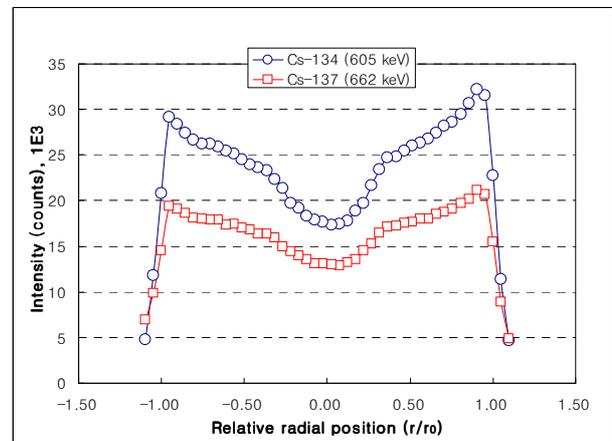
Figure 1. Cs-134 and Cs-137 profiles across a fuel pellet
