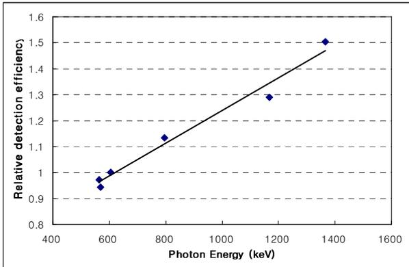
Figure 2. Relative detection efficiency measured by the axial gamma scanning
