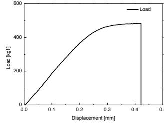
Fig. 7 Example of load-displacement curve from test.
