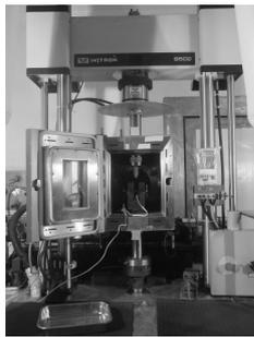
Fig. 5 Universal testing machine in hot cell.
