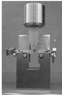
Fig. 6 Jig for PCVN specimen.
