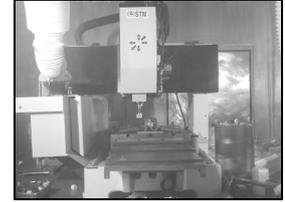
Fig. 1 Broken Charpy specimen Fig. 2 CNC milling machine in hot cell.
