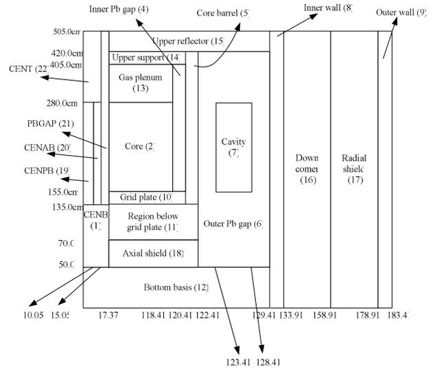
Figure 1. Configuration of the ENHS reactor with P/D=1.44; not to scale.
