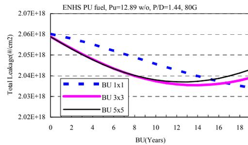
Figure 5. Total Leakage versus Burnup
