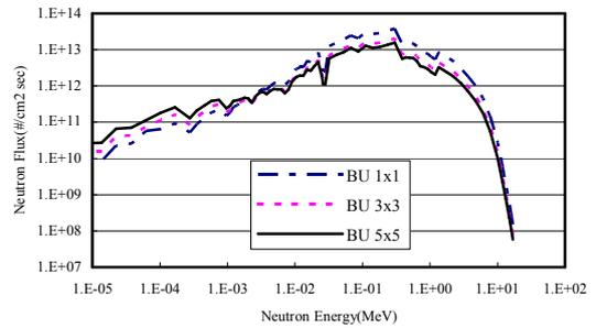
Figure 4. Comparison of neutron spectrum at the outer bottom of core, BOC
