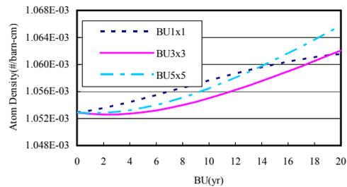
Figure 6. Total Pu Atom Density versus Burnup
