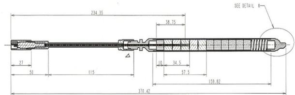
Figure 2. Design of the instrumented mini-element
