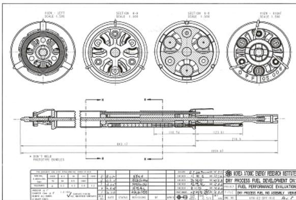
Figure 1. Design of the instrumentation rig
