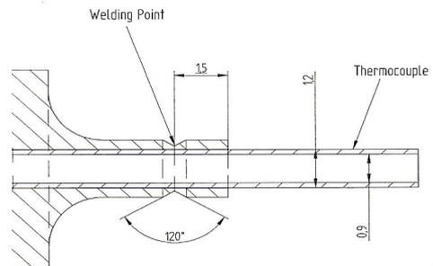
Figure 3. Laser micro-welding of thermocouple
