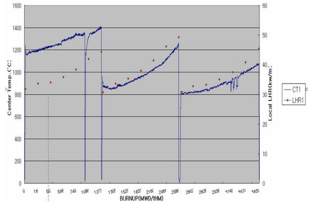
Figure 6. Pellet centerline temperature(#1) acquired by DAS and Linear Heat Rate
