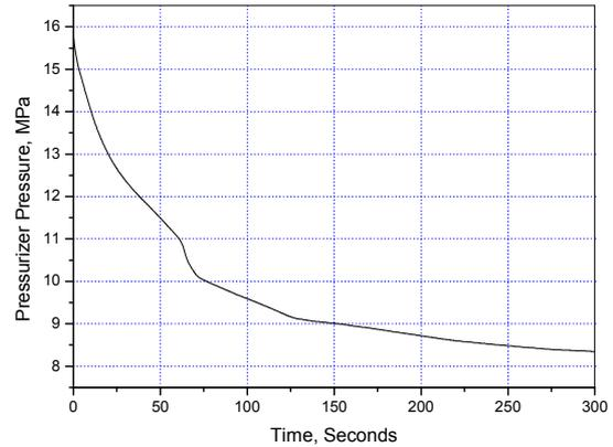
Figure 2 Pressurizer pressure change of SGMPB
