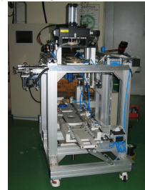
Fig 2. Photography of the multi-pin welding machine.
