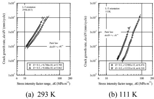
Fig. 1 The effect of stress ratio on the fatigue crack growth rate
