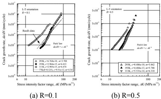
Fig. 2 The effect of low temperature on the fatigue crack growth rate
