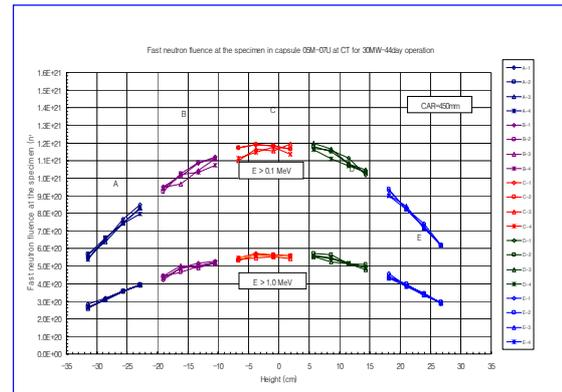
Figure 4. The axial distribution of the fast neutron fluence of the specimens in 05M-07U capsule
