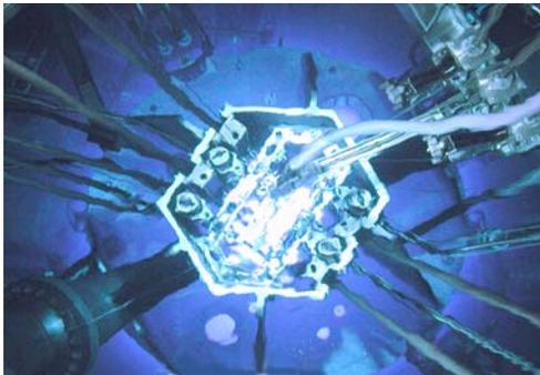
Figure 3. Reactor core during an irradiation test in HANARO
