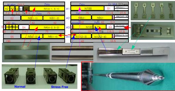
Figure 2. Specimen configuration in the capsule
