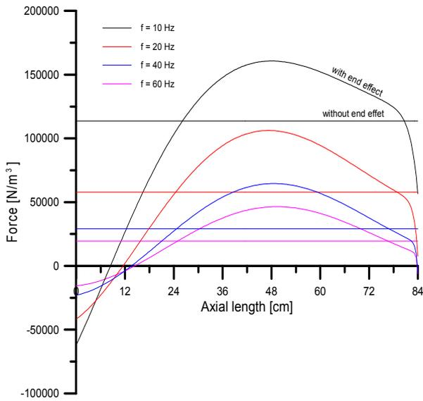
Fig. 3. Distribution of Force according to Axial Length of the Pump (Pump of diameter = 10 cm and length = 84 cm with 40 l/min)
