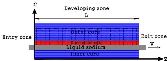
Fig. 2. Mathematical Model of the EM Pump of the Annular Type
