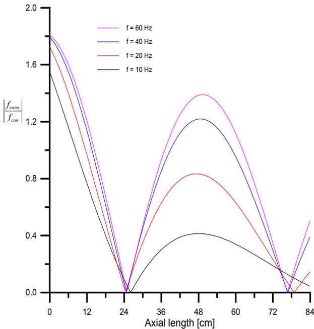
Fig. 4. Ratio of Entry End Effect to Conventional Force
