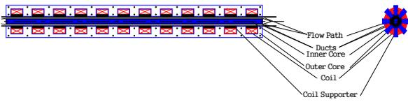
Fig. 1 Cross-Sectional View of the Annular Linear Induction EM Pump
