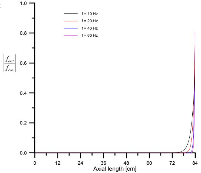
Fig. 5. Ratio of Exit End Effect to Conventional Force
