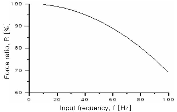
Fig. 6. Ratio of Both Forces in Case with and without End Effect according to Frequency Change
