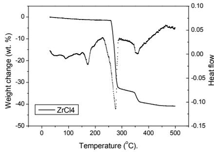
Fig. 2. TG-DTA result of ZrCl<sub>4</sub> powder.
