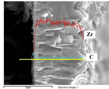
Fig. 5. EDS result of ZrC film with various vaporizer temperatures 300°C and amount of ZrCl<sub>4</sub> powder of 20g.
