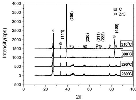
Fig. 3. XRD patterns of ZrC films with various vaporizer temperatures.
