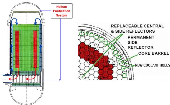
Figure 3. Inlet Flow Configuration of H2-MHR<sup>[4]</sup>
