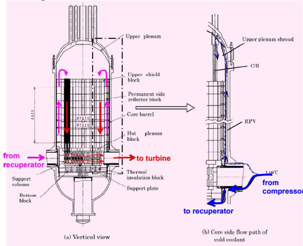
Figure 2. Flow path in RPV of GTHTR<sup>[3]</sup>
